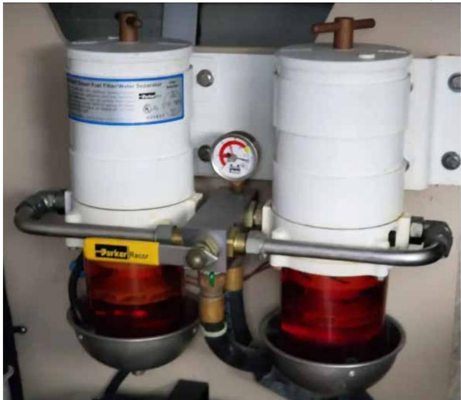
unfiltered fuel to go directly into the fuel injection pump and injectors. Changing the primary and secondary fuel filters at regular intervals is important and monitoring engine performance is an effective way to know when a fuel filter has become restricted
