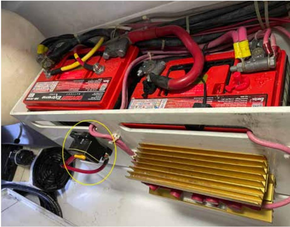
ship's battery or a dedicated battery and not tied into the boat's electrical panel or other junction etc. Imagine retrieving two dredges at the same time, pulling up to 60 amps instantly can overload existing boat circuits.
