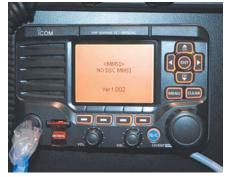
For older radios not having a test call capability, testing can only be performed by using a routine individual call to a fellow boater. Under no circumstances shall a DSC distress alert be sent to test your radio. It is a violation of the rules and can result in heavy fines "
